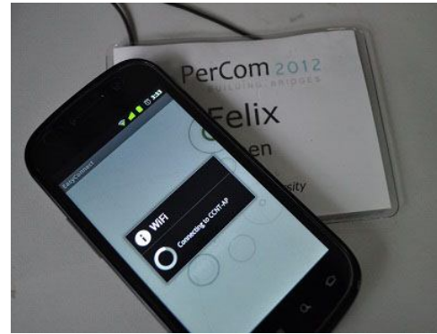
Figure 3. Touch&Connect: Connecting to WiFi network by touching the smartphone with the conference badge.
