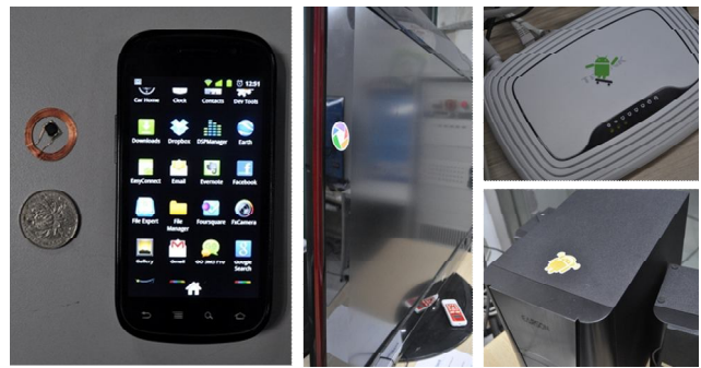
Figure 1. The smartphone (Google Nexus S) and NFC tag, as well as three NFC tagged devices (a TV, a WiFi router, and a speaker).
