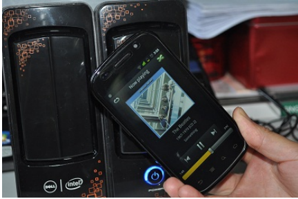
Figure 7. Touch&Listen: Streaming music seamlessly from phone to Bluetooth speakers by touching them
